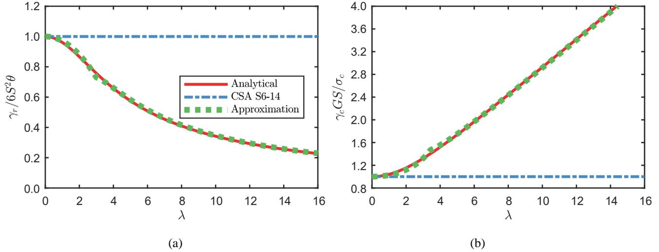
Figure 6: Comparison of the analytical solution to the proposed approximation and the CHBDC equation for (a)  $\gamma_r$  and (b)  $\gamma_c$  of a circular pad
