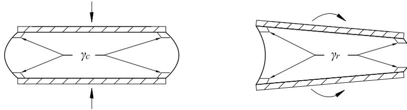
Figure 2: Location of the maximum shear stress due to compression and rotation for a single layer of elastomer between reinforcement layers
