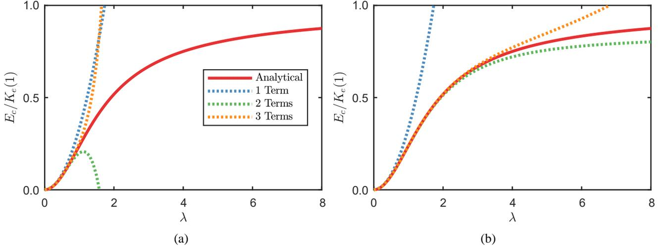
Figure 4: Comparison of the analytical solution for  $E_c$  to the truncated Taylor series expansion of the (a) original expression and (b) inverted expression.
