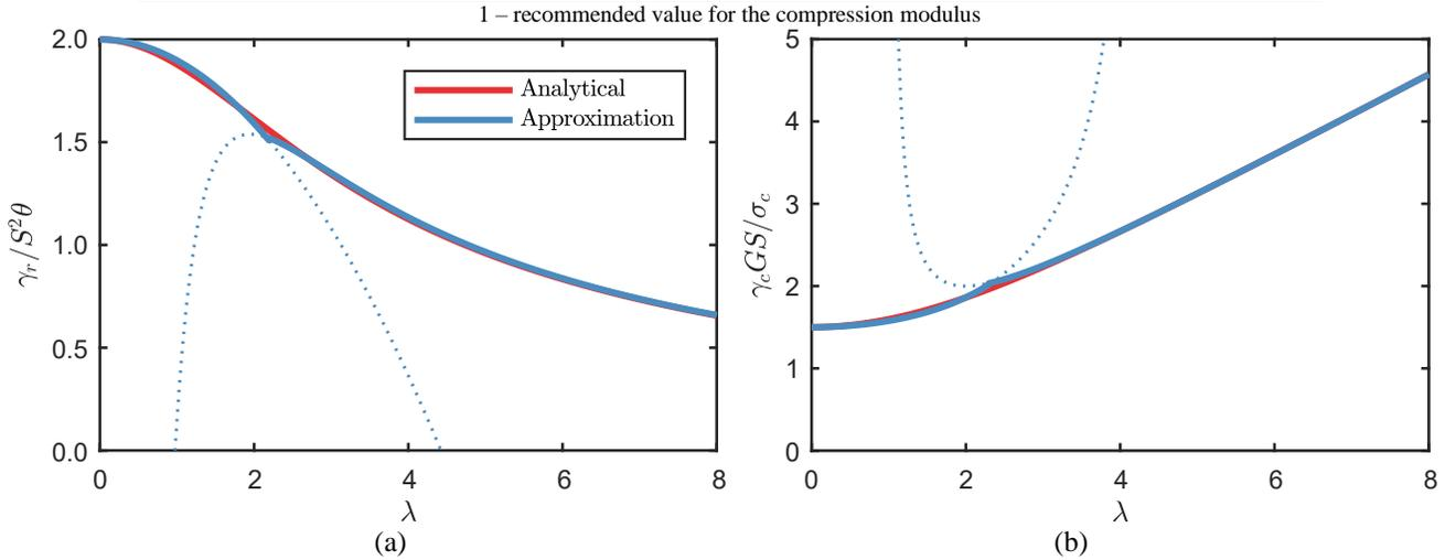
Figure 5: Comparison of the analytical solution to the proposed approximation for (a)  $\gamma_r$  and (b)  $\gamma_c$  of an infinite strip pad
