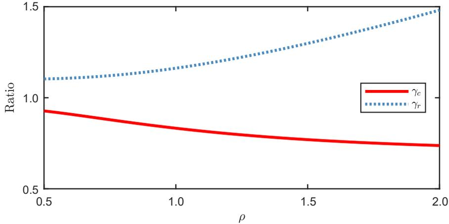
Figure 3: Ratio of the shear strain determined from the CHBDC to the analytical solution assuming an incompressible elastomer and inextensible reinforcement.
